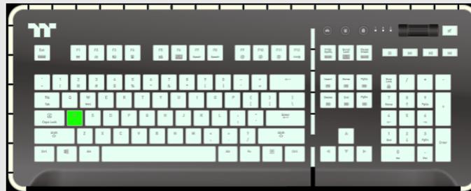
✘ Press and hold a key which has been assigned a macro for more than 3 seconds to erase the saved macro.
